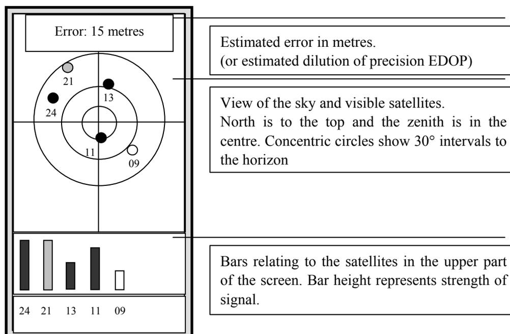
Figure 6-2 Basic GPS screen layout.
