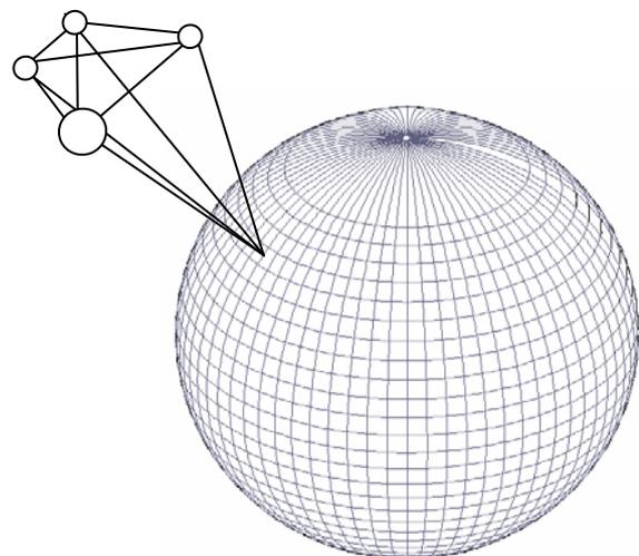
Figure 6-10 Basic Trigonometry - Four Satellites.
