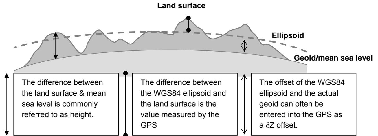
Figure 6-16 Offsets between geoid, ellipsoidal and land surface.
