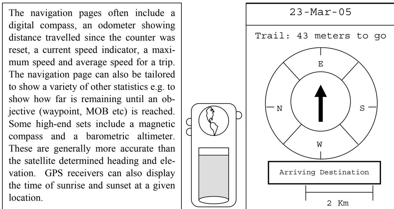
Figure 6-5 Basic GPS Man Over Board or Track Back features.
