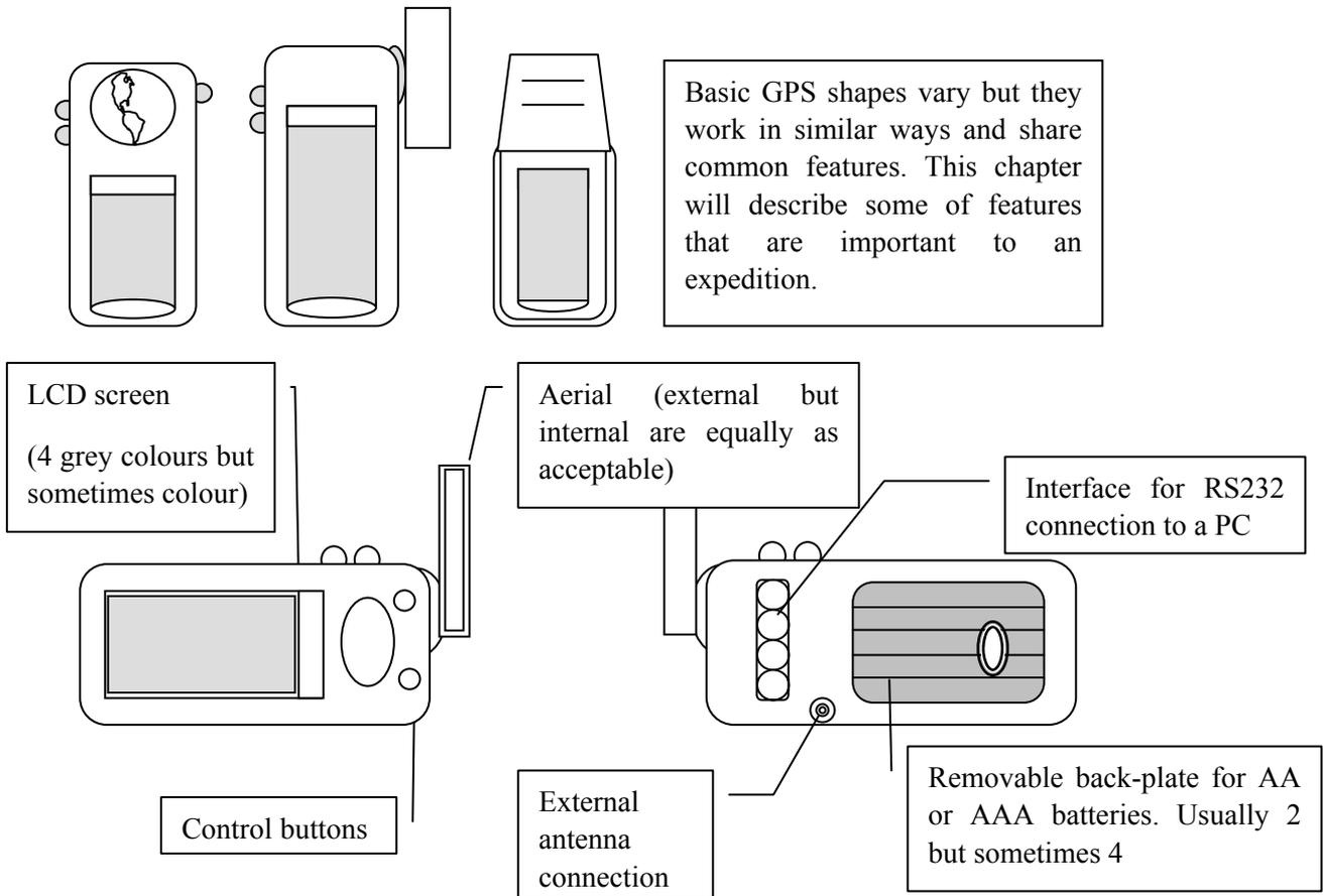
Figure 6-1 A basic guide to GPS models.
