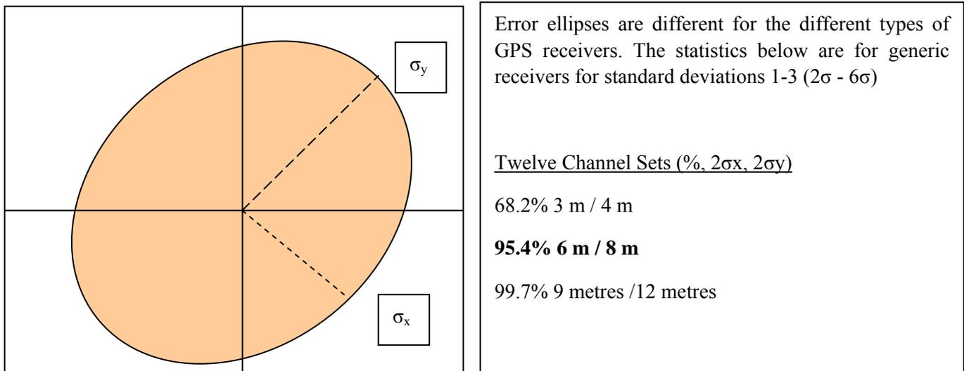
Figure 6-13 Error ellipse for 12 channel GPS.
