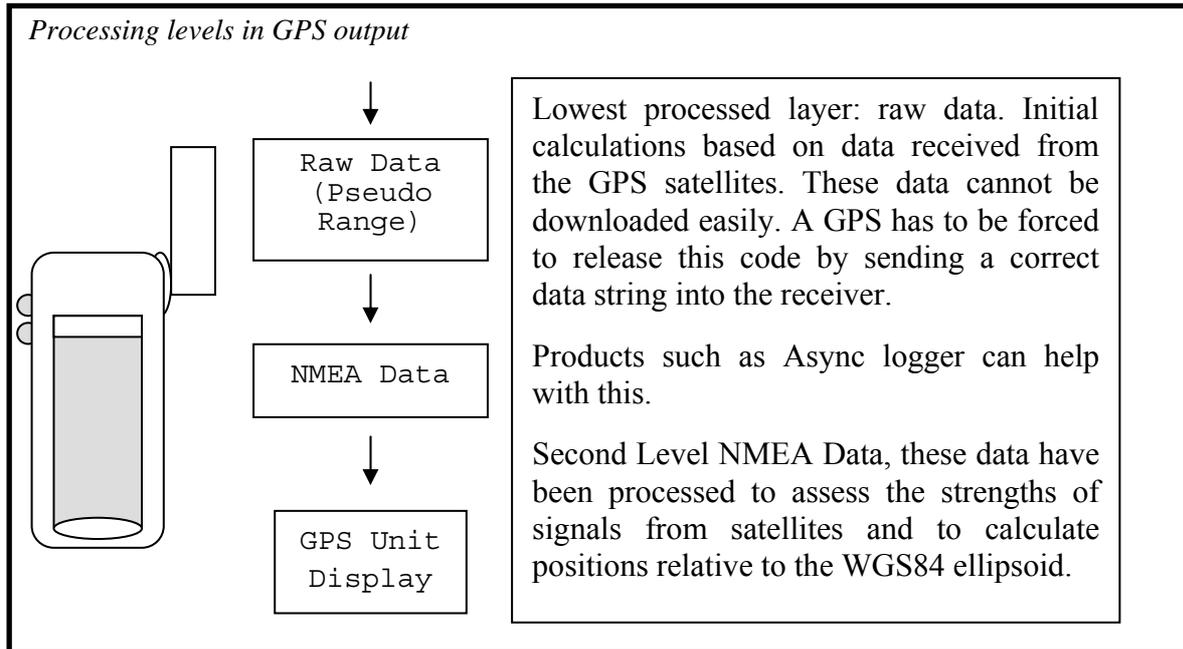
Figure 6-17 Processing tiers in the GPS positioning architecture.
