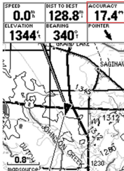
Figure 4. Example Map Screen – with accuracy highlighted in a red box.
